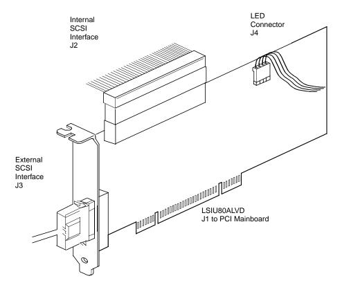
Step 6. Carefully insert edge connector J1 (see Figure 2.1) of the host adapter into the PCI slot. Make sure the edge connector is properly aligned before pressing the board into place as shown in Figure 2.2.
